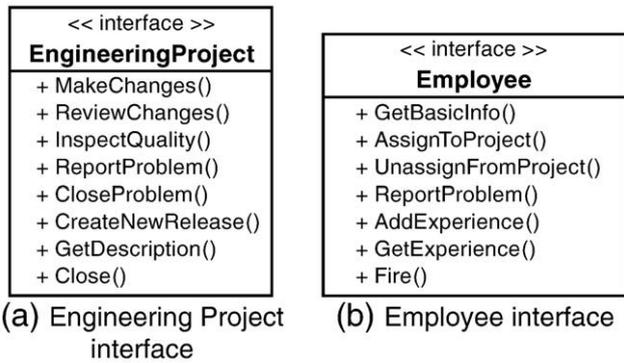
Fig. 5. Example COM+ interfaces.
