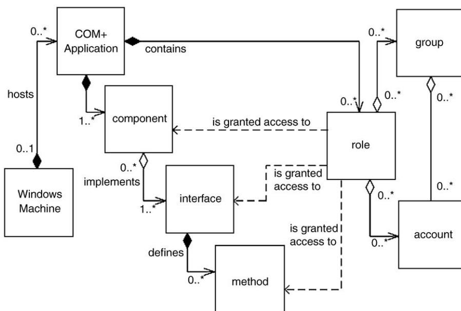
Fig. 4. UML model of COM+ access control architecture.
