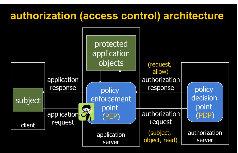
this architecture is based on the point-to-point model, used by IBM Access Manager, Entrust GetAccess, CA SiteMinder, etc.
