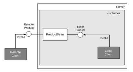
Figure 3.1: Basic parts of EJB architecture for an example Enterprise Java Bean Product
