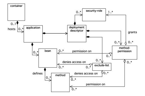
Figure 3.4: Relationships among the sections of deployment descriptor used for expressing access control policy and the elements of an EJB application
