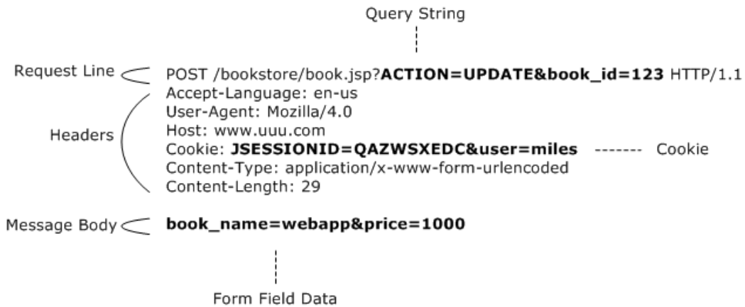
Figure 4.1: Structure of an HTTP request and sources of name-value pairs
